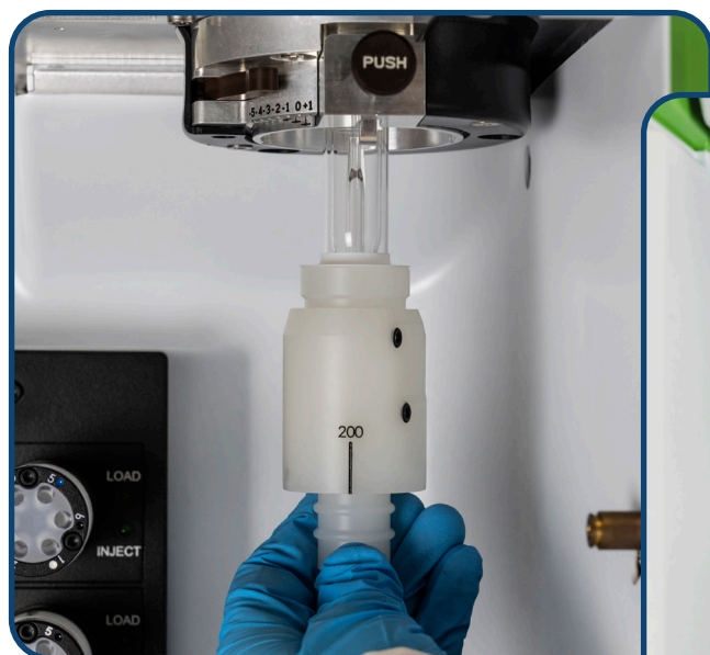
Installing a ZipTorch on Avio 200
